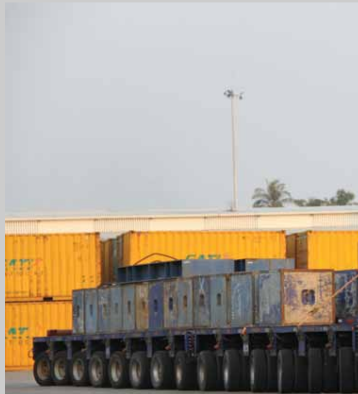
The 14-axle heavy trailer used in the operation. Photo: The
